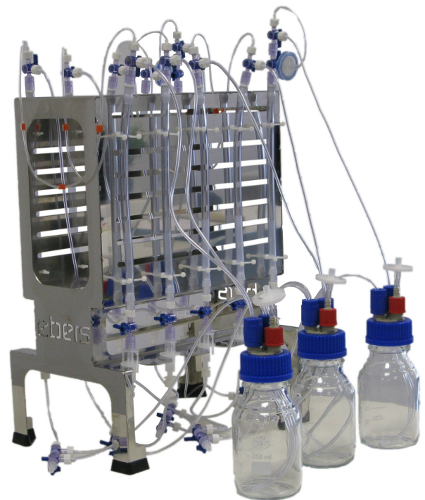
Figure 1. Seeding rack with pre-built circuits and P3D chambers
