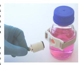
Optical readers can measure through almost any non-colored transparent thin wall in a noninvasive mode. Moreover, the software allows operating up to ten readers simultaneously and log the measurements for post-processing through a single PC connection.
