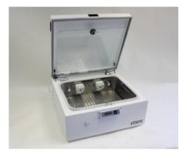
The TEB500 series is equipped with  $CO_2$  and  $O_2$  controls in its standard version and allows the user to:
