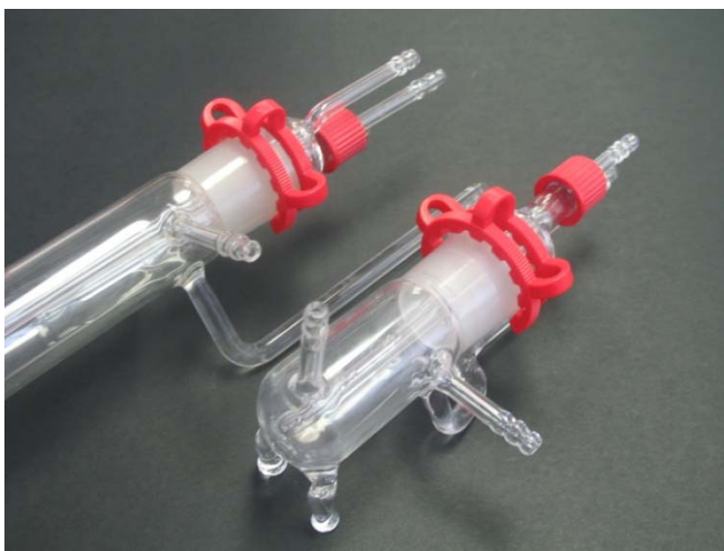
Figure 2. Culture chamber for vascular applications
